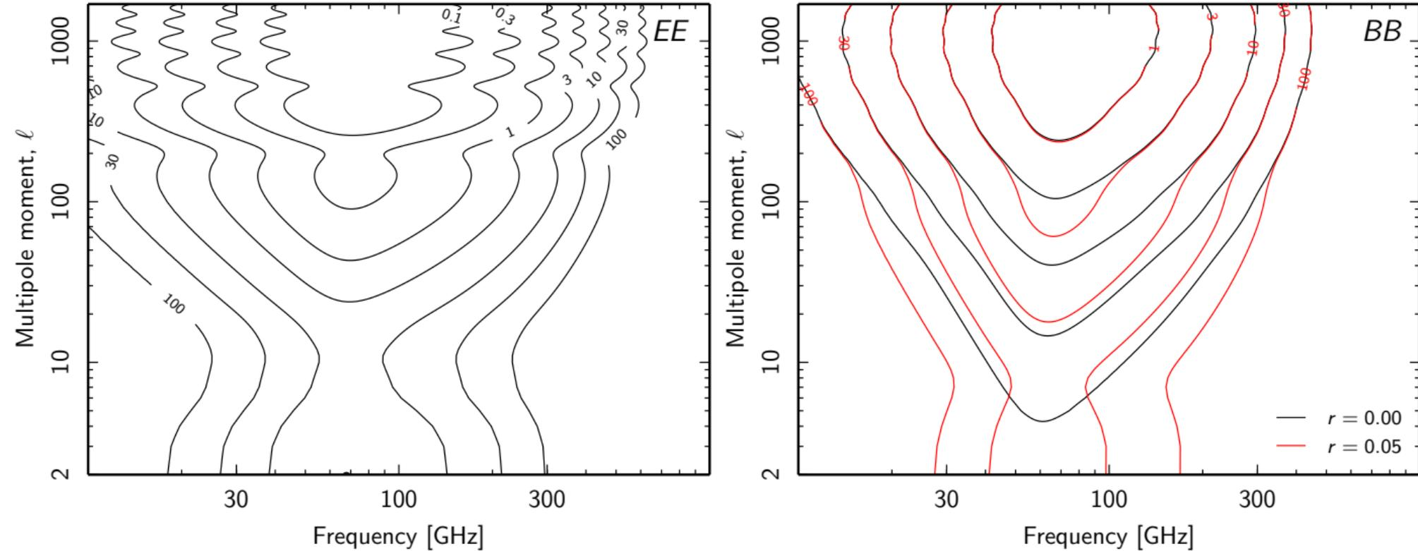
**Fig. 45.** Amplitude ratio between total polarized foregrounds and CMB as a function of both multipole moment and frequency, defined by  $f(\ell, \nu) = [C_\ell^{\text{fg}}(\nu)/C_\ell^{\text{CMB}}]^{1/2}$ , as defined Eq. 22 with parameters derived from 73 % of the sky. The left and right panels show the  $EE$  and  $BB$  spectra, and the black and red contours in the latter corresponds to tensor-to-scalar ratios of  $r = 0.0$  and  $0.05$ , respectively.
