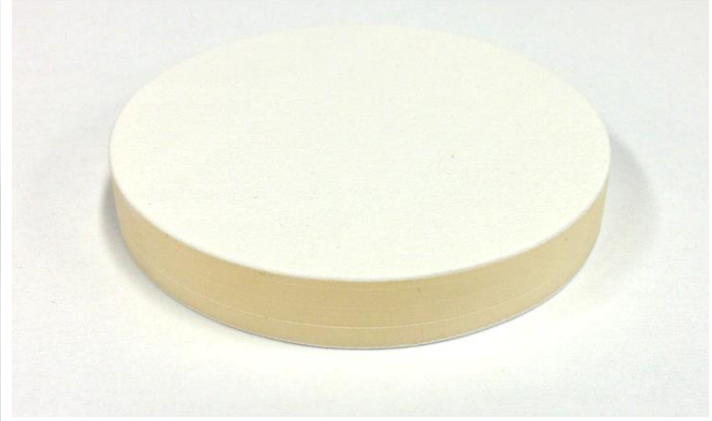
Alumina coated with two layer thermal sprayed layer + Teflon outer layer, room temp
